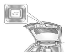
Pressing and releasing the power liftgate button on the liftgate adjacent to the latch to close the liftgate. Pressing any button that operates the power liftgate, or the touchpad while the liftgate is moving, stops it. Pressing the button or RKE again reverses the direction. There is a minimum that the power liftgate must already be open for the system to hold it open. If movement is stopped below that minimum, the liftgate closes.
